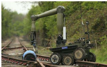
Bomb disposal robots have been deployed as a first line of response to ensure safety of our army personnels.
