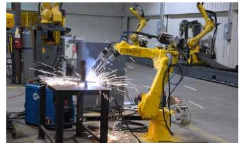
Robots performing dangerous welding work with precision.
